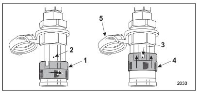
Figure 3-34 Quick Connect Locking Collar
